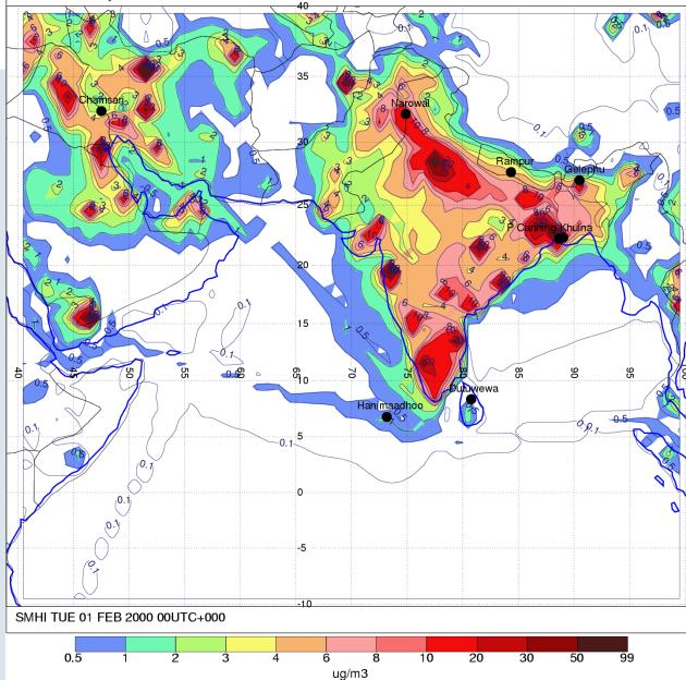
Modelled near-surface SO<sub>2</sub> concentration in Malé domain during January 2000 using EDGAR emissions valid for 1995
